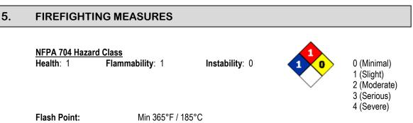
Flash Point Test Method: Cleveland Open Cup (COC), ASTM D92
